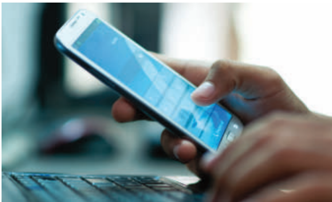
Fig. 1: By detecting user proximity, the smartphone can turn off the display backlight and the touch screen when the smartphone is held up to the user's ear saving battery life and helping to prevent inadvertent touch screen interaction. (All figures courtesy of AMS ag)
